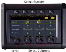
Use the left knob to scroll up and down the menu and the others to change the value of the variable within each axis.
